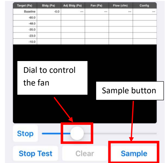
Image of the dial to control the fan and the sampling button
