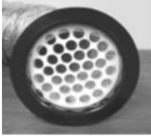
Figure 2 Duct Blaster Flow Conditioner
