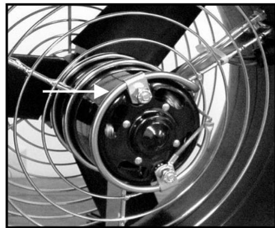
Duct blaster flow sensor
